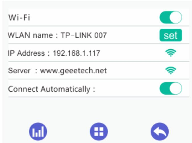
Step 9. Go back to the App, click [OK] to enter the home page. The status on the homepage displays that the printer is on-line. Till here, the configuration between App and the printer is finished. Now you can print and control the printing via App.
