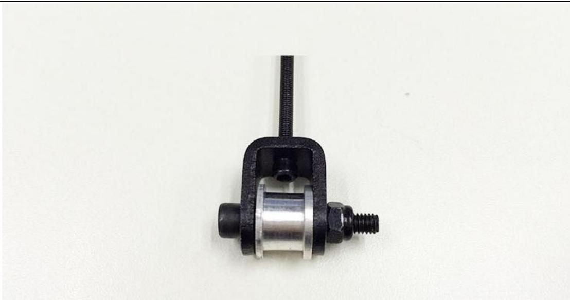
\*Note: Do not screw it too tightly as it may restrict the free movement of the drive wheel. It is important that you leave enough room for the wheel to turn freely.
