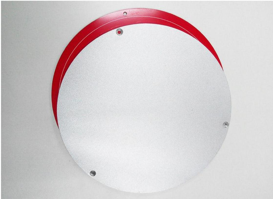
Step 2. Thread the M3x30mm Hex sunk screw (#15) through the building platform (M5) and heat-bed (#56), add washers (#5) and spring (#30); the assembly should now look like this:
