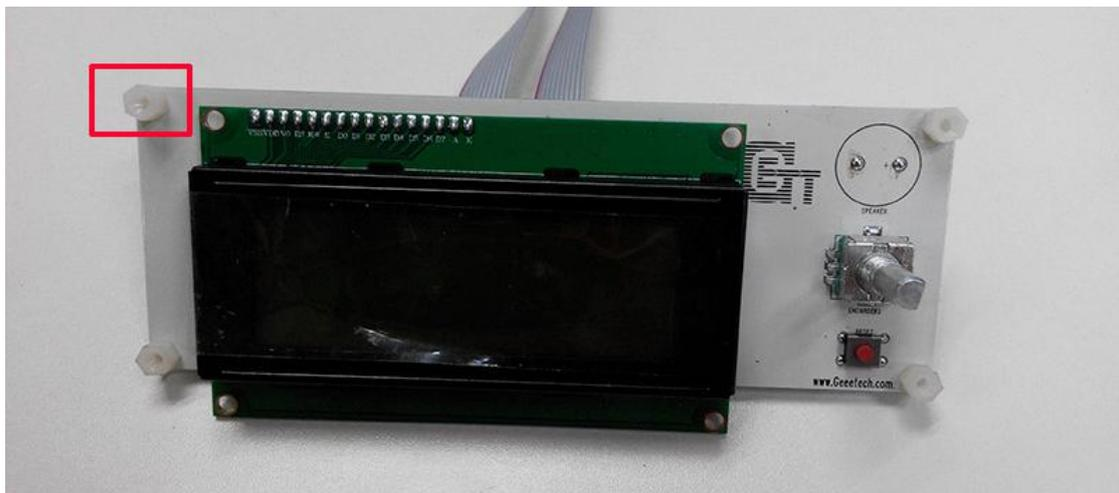
Step 3. Assemble the LCD frame (#A8) and LCD2004 (#49) with 4 M3 x 12 Screws (#20) and washers (#5).
