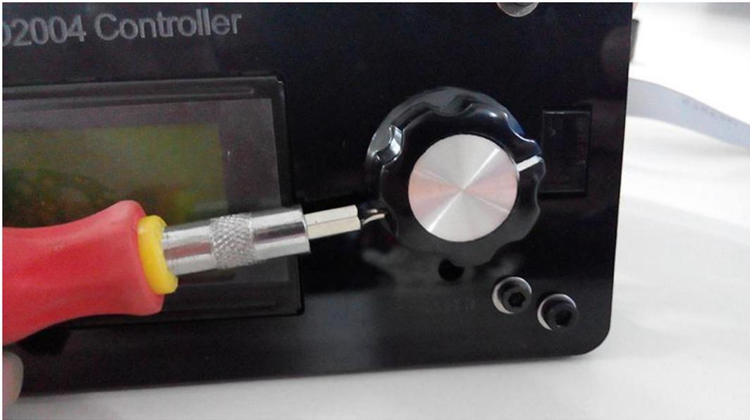
Step 5. Mount the assembled LCD kit onto the base plate. Screw it up with 2 M3 x 16 screws (#21), M3 square nuts (#13) and washers (#5).
