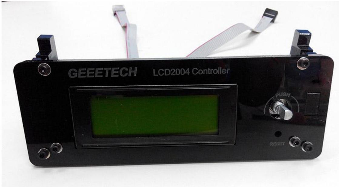
Step 4. Install the knob over the protruding stalk and screw it in place with the screw located in the hole.
